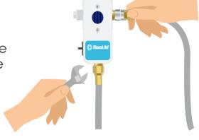
4-The other end of the dispensing gun hose can now be screwed onto the dispensing gun.
