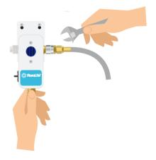
2-The other end of the water source hose is a standard fitting that can be installed or adapted to any water faucet/connection.
